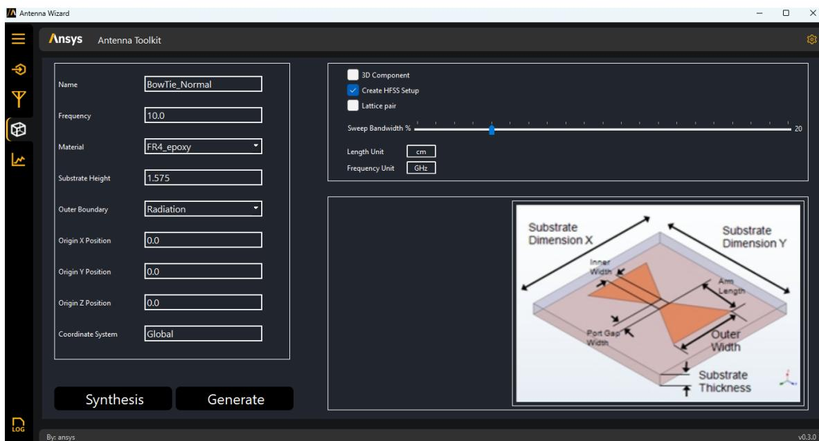
You have two options: **Synthesis** and **Generate**. The **Generate** button is unavailable if the wizard is not connected to AEDT.
